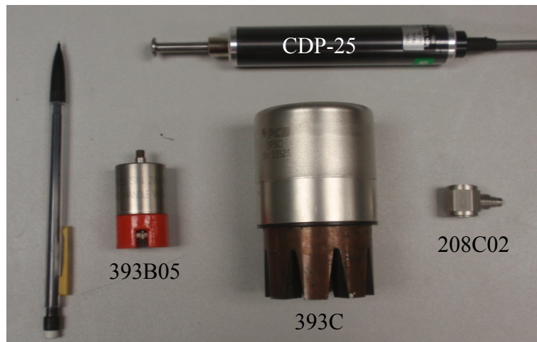
Figure 6.6. Photograph of sensors used in laboratory testing. (Photo by EVF, dynamics lab, 7/9/13)
