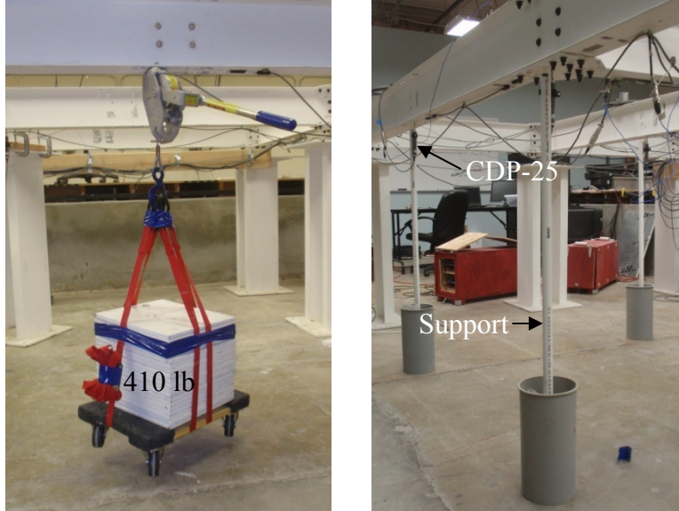
Figure 6.25. Photographs of suspended load and displacement transducers used for static load testing. (Photos by EVF, dynamics lab, 7/9/13)
