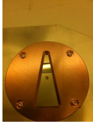
Figure 3.11 (b) Front side of loaded piece cassette (Thach Pham, January 2013, University of Arkansas)
