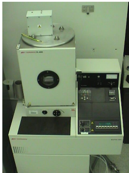
Figure 3.16 Thermal evaporator Edward 306T (Thach Pham, July 2013, University of Arkansas)
