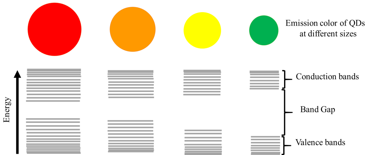
Figure 1.1a: Evolution of quantum dots color, bands and band gaps as size decreases showing quantum confinement effect.
