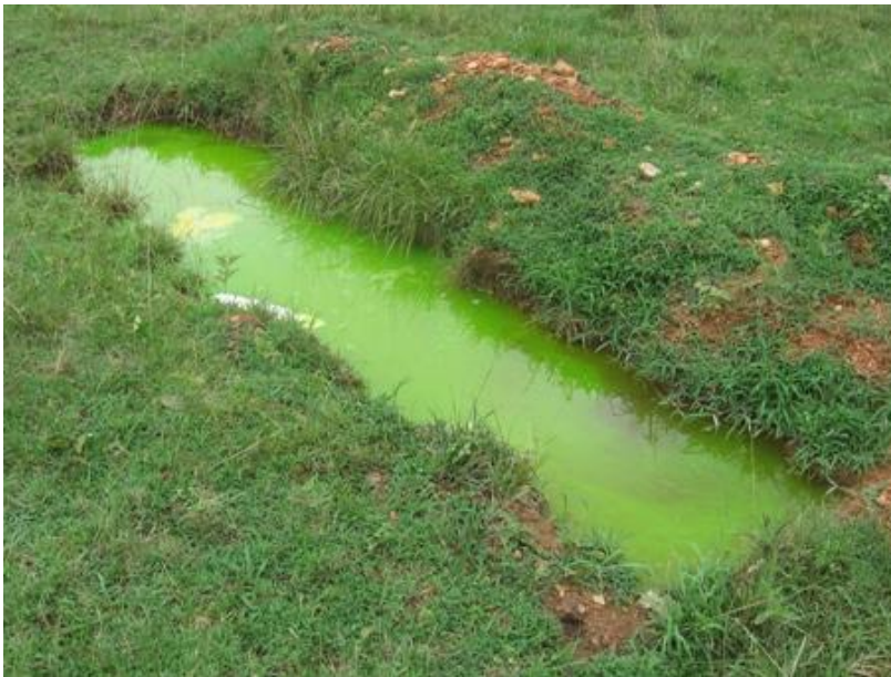
Figure 4-5 Dye injected into trenches situated on the pasture inside the instrumented plot. The trench in the upper photograph is on the east side of the plot, the other trench is on the west side. (Photo by author)
