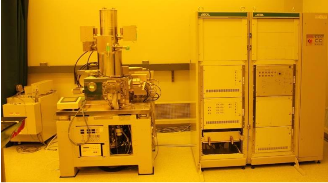
Fig. 2-7 JEOL JBX-5500ZD EBL writer is located in High Density Electronics Center (HiDEC) at University of Arkansas, Fayetteville [43].
