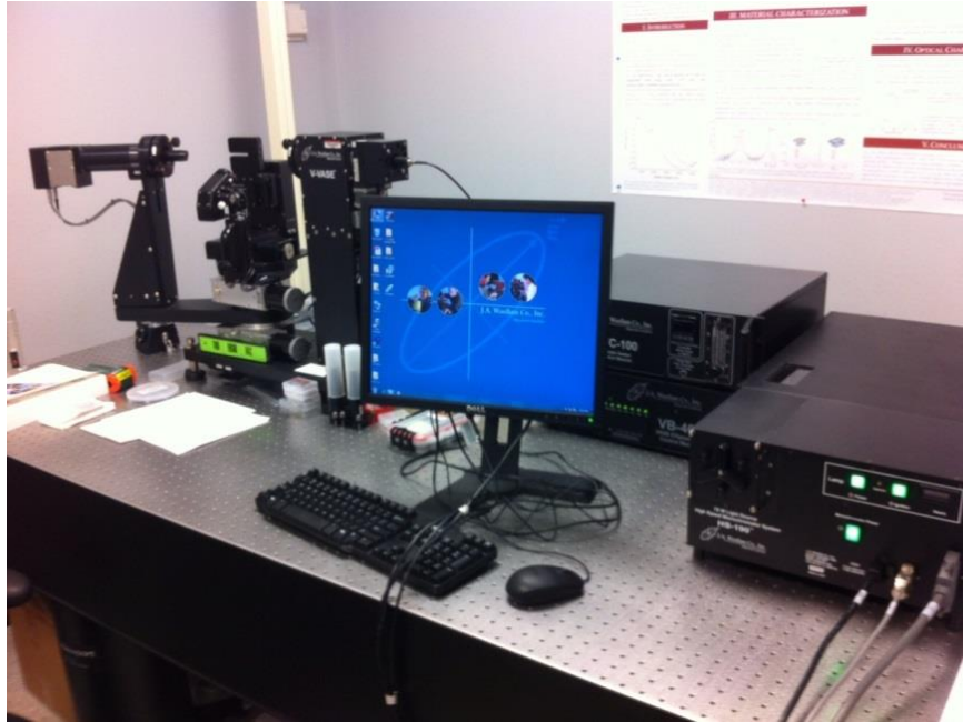
Fig. 4-4 The VASE variable angle spectroscopic ellipsometry system is shown in operation mode (this picture is taken by author at Dr. Shui-Qing Yu's lab on March 10 2014).
