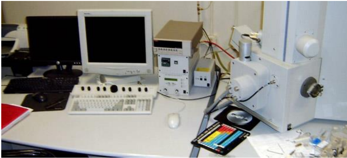
Fig. 2-5 The Philips XL30 ESEM modified EBL writer is shown integrated with Nanometer Pattern Generation System (NPGS) [42].
