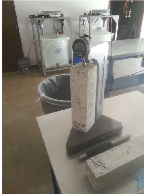
Figure 2-4: ASR prism being tested for expansion.
