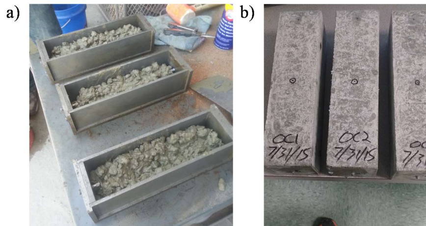
Figure 2-1: a) Casting of prisms and b) cured prisms.
