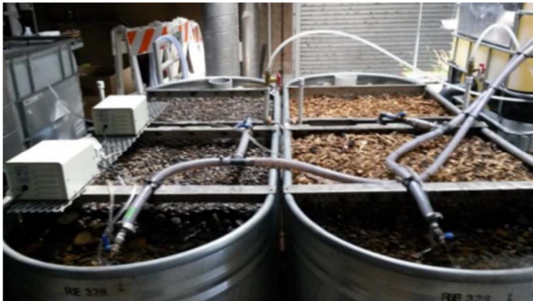
Figure 10: Photograph of a denitrification bioreactor experiment executed by Clean Water Services in Hillsboro, Oregon ( Clean Water Services Denitrification Pilot Reactors ).
