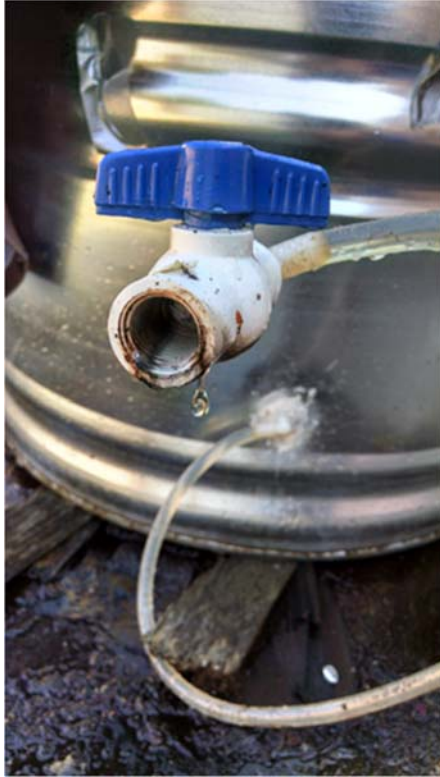
Figure 8: Photograph of the valve system used to control the effluent flow. This was responsible for releasing 40 gallons per day.
