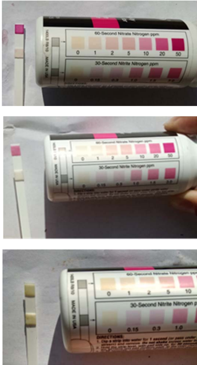
Figure 19: Photographs of testing strips used to measure nitrates in the effluent. The top photograph shows Day One with a high nitrate concentration. The middle photo shows Day Three with a reduced nitrate concentration. The bottom photo shows the results we received from Day Five until we stopped testing.
