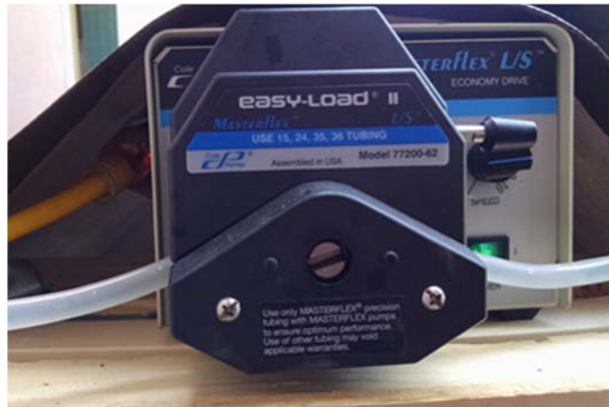
Figure 7: Photograph of the pump used during this project. This pump was responsible for pumping 40 gallons per day into the system.
