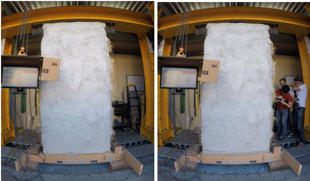
Figure 12: Welded-18 wall at (a) 1.28” lateral displacement with lateral load 998 lbs and (b) 2.88” lateral displacement with lateral load 1567 lbs. These photos were taken during a leading cycle.
