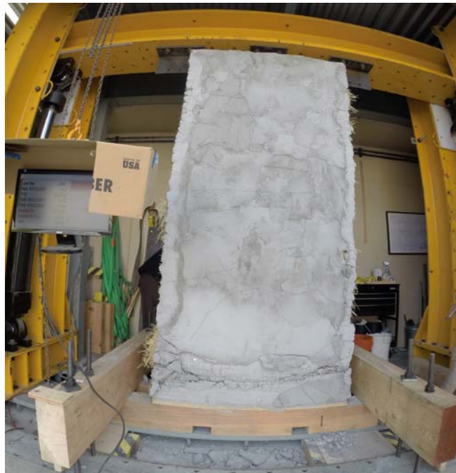
Figure 26: Welded-14 at 3.70” lateral displacement with load 229 lbs. Taken during a trailing cycle.
