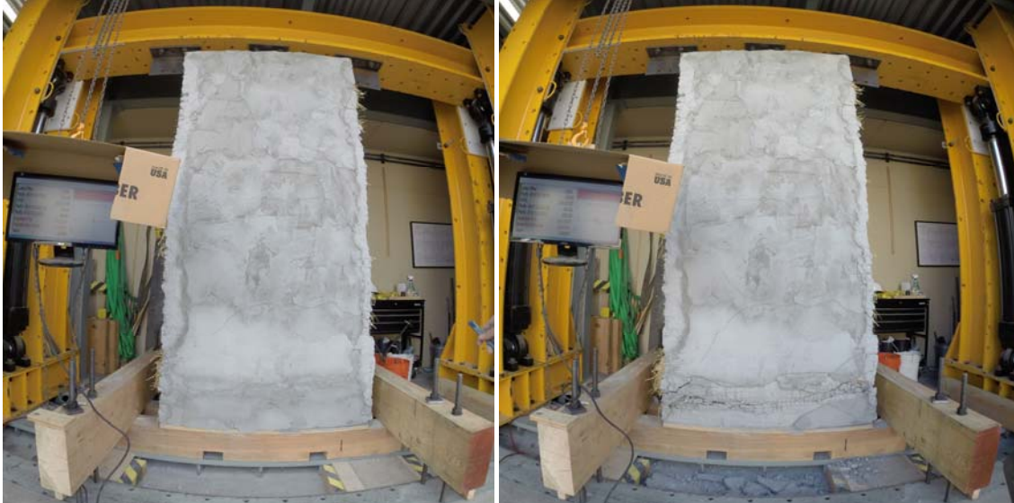
Figure 25 Welded-14 at (a) 1.17” lateral displacement and load 1704 lbs and (b) 3.26” lateral displacement with load 520 lbs. Both images were taken during a leading cycle.
