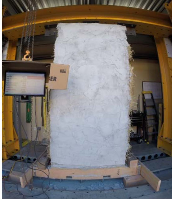
Figure 13: Welded-18 wall at 4.3” lateral displacement with lateral load 521 lbs. Taken during a leading cycle.
