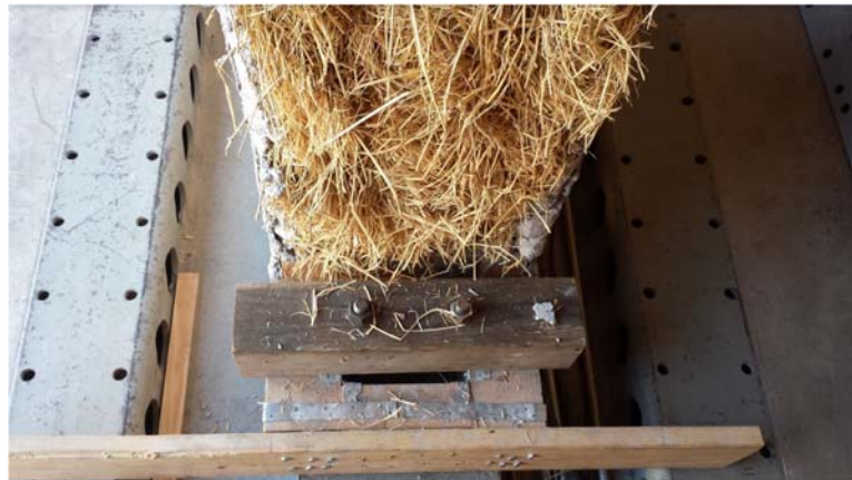
Figure 10: Connection of the base of the wall to the floor of the test frame.
