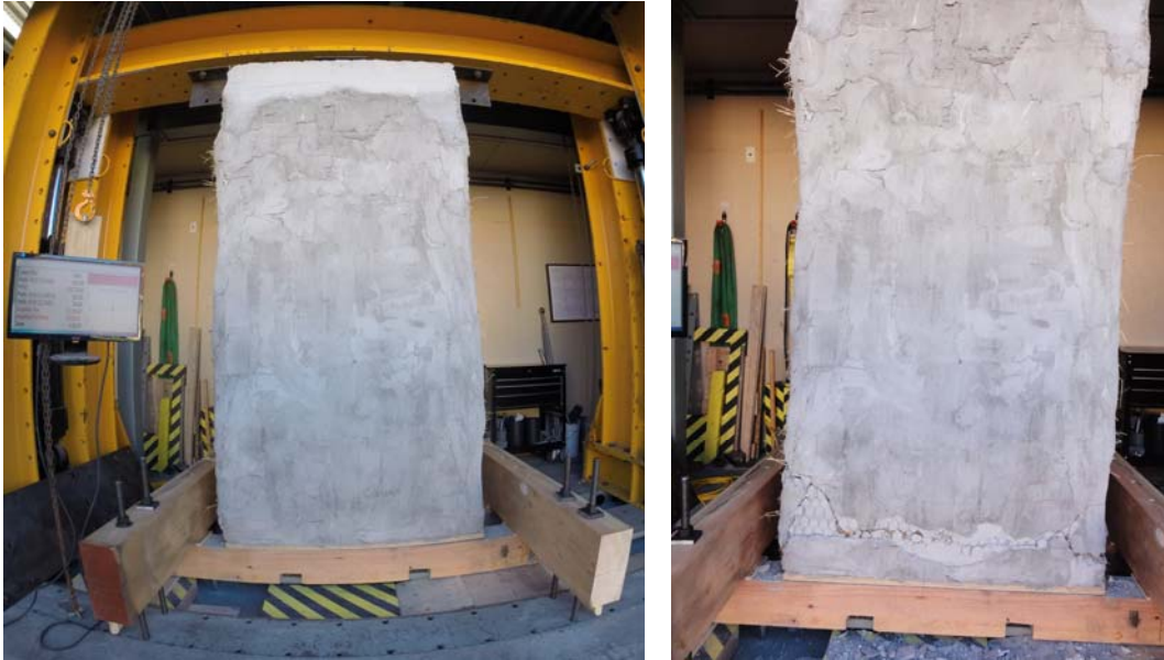
Figure 19: Woven-18 wall at (a) 1.06” lateral displacement with lateral load 1402 lbs and (b) approx. 3” lateral displacement at an unspecified lateral load. Figure 19(a) was taken during a leading cycle, and Figure 19(b) was taken during a trailing cycle.
