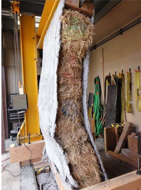
Figure 31: Side view of the Welded-9 wall buckling during the vertical test.
