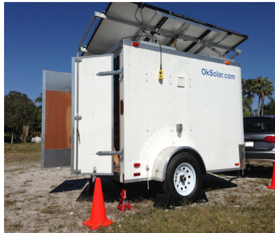
Figure 23. Military Grade Solar Transportable Modular Power Unit, OkSolar.com.
