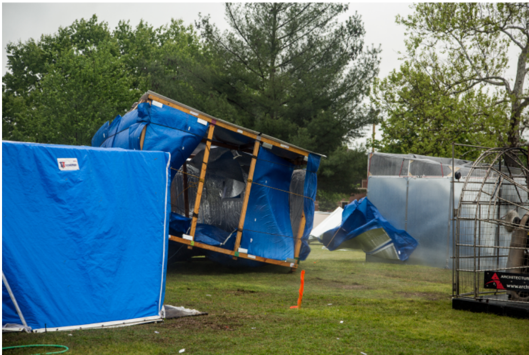
Figure 25. Prototype at failure during wind test
