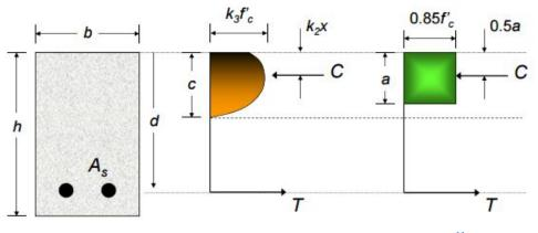
**Figure 7: Diagram of a compression stress block**<sup>11</sup>.
