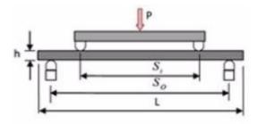
Figure 6: Diagram of a four-point load test.
