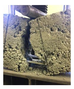
Figure 12: Failed beam with fish netting reinforcement.
