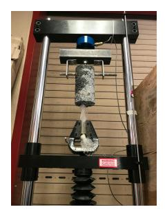
Figure 14: Testing Apparatus for pull-out test using fish netting.
