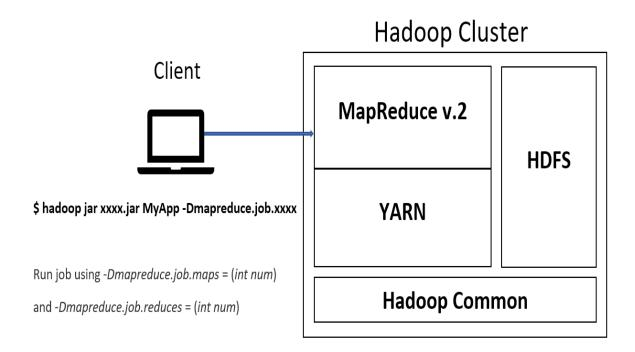
Fig. 8 Allocating Task Resources to Sample Executions on the Target Hadoop Cluster.
