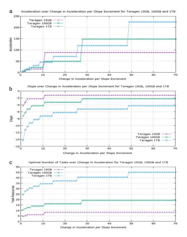
Fig. 14 The optimal number of tasks for Teragen 10 GB, 100 GB, and 1 TB workloads are identified by the major plateaus lasting at least eight increments on the graphs. The algorithm searches for break points in the changes in acceleration and outputs: (a) recommended acceleration, (b) corresponding slope and (c) task resources versus change in acceleration per slope increment.
