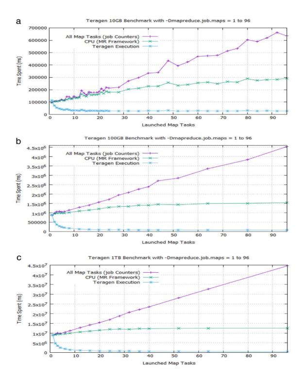
Fig. 7 Graphs of time spent by all map tasks, CPU, and Teragen execution versus number of launched map tasks. The runtime elbow curves of Teragen (a) 10 GB, (b) 100 GB and (c) 1 TB workloads plotted at different y-axis scales all appear to have the best trade-off points for performance efficiency at around 10 map tasks. But that is refuted by our algorithm as a visual misperception of different granularities at low magnification.
