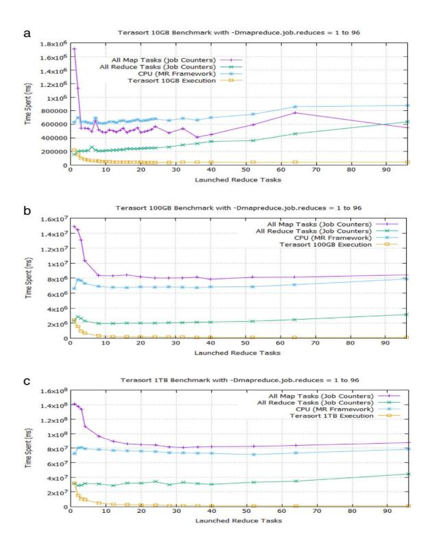
Fig. 10 Graphs of time spent by all map tasks, all reduce tasks, CPU, and Terasort execution versus number of launched reduce tasks. The runtime elbow curves of Terasort (a) 10 GB, (b) 100 GB and (c) 1 TB workloads plotted at different y-axis scales all appear to have the best trade-off points for performance efficiency at around 10 reduce tasks. But that is disproved by our algorithm as a visual misperception of different granularities at low magnification.
