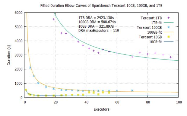
Fig. 25 Fitted runtime vs. executors' elbow curves of SparkBench Terasort 10GB, 100GB, and 1TB of data, and their runtimes with Dynamic Resource Allocation (DRA) enabled.
