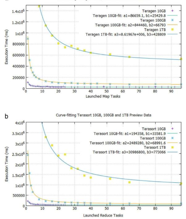
Fig. 12 Fitted runtime elbow curves of (a) Teragen and (b) Terasort 10 GB, 100 GB, and 1 TB workloads versus number of launched map/reduce tasks, and their fit parameters a and b in the graph function f(x) = (a/x) + b.
