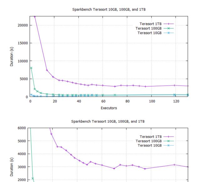
Fig. 23 Plots of Preview data of duration vs. executors of SparkBench Terasort 10GB, 100GB and 1TB of data at different vertical scales.
