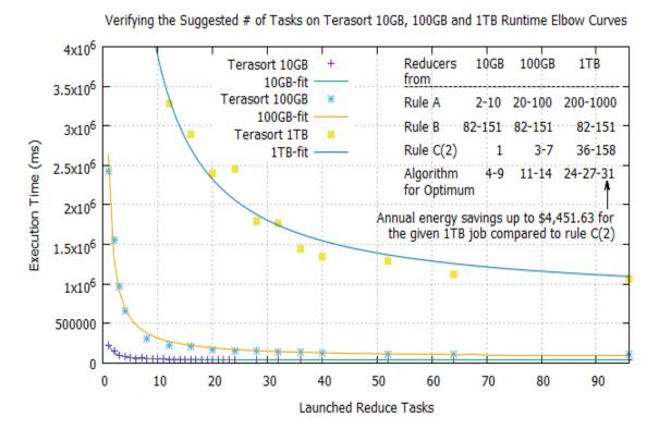
Fig. 17 Fitted elbow curves of Terasort 10 GB, 100 GB, and 1 TB workloads from sampled executions verify the accuracy of our algorithm for optimal resource provisioning in contrast to the unreliable number of reducers calculated from three popular rules of thumb (A, B, and C(2)), which could lead to significant waste of computing resources and energy.
