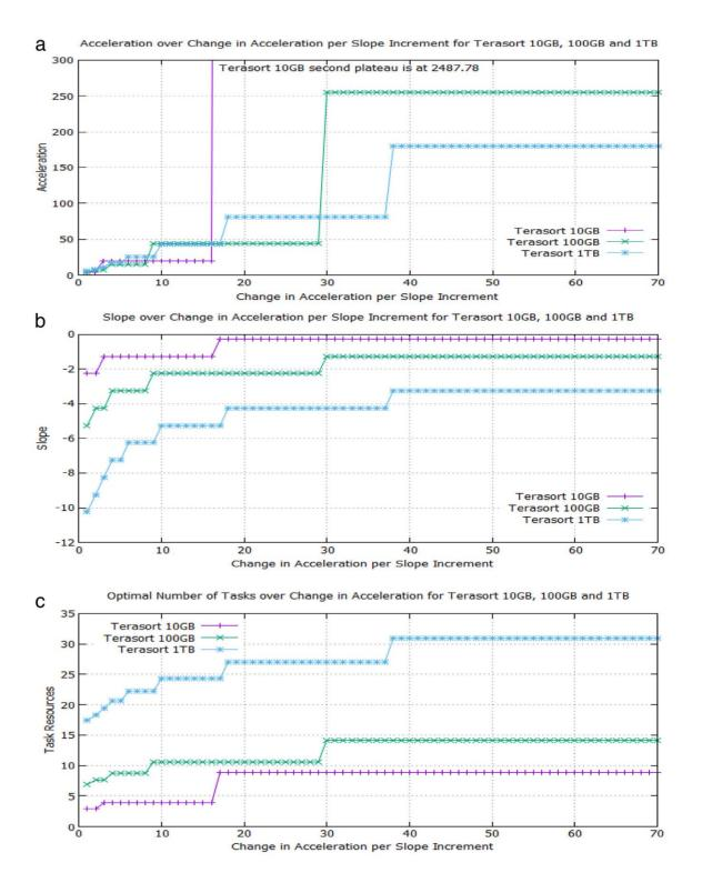
Fig. 16 The optimal numbers of tasks for Terasort 10 GB, 100 GB, and 1 TB workloads are identified by the major plateaus lasting at least eight increments on the graphs. The algorithm searches for break points in the changes in acceleration and outputs: (a) recommended acceleration, (b) corresponding slope and (c) task resources versus change in acceleration per slope increment.
