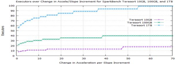
Fig. 27 The optimal numbers of executors for Spark-Bench Terasort 10 GB, 100 GB, and 1 TB workloads are identified by the major plateaus lasting at least seven increments on the graphs. The algorithm searches for break points in the changes in acceleration and outputs: (a) recommended acceleration, (b) corresponding slope and (c) executors versus change in acceleration per slope increment.
