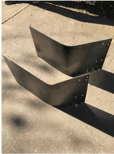
Figure 28: Deformed Plates after Impact Test
