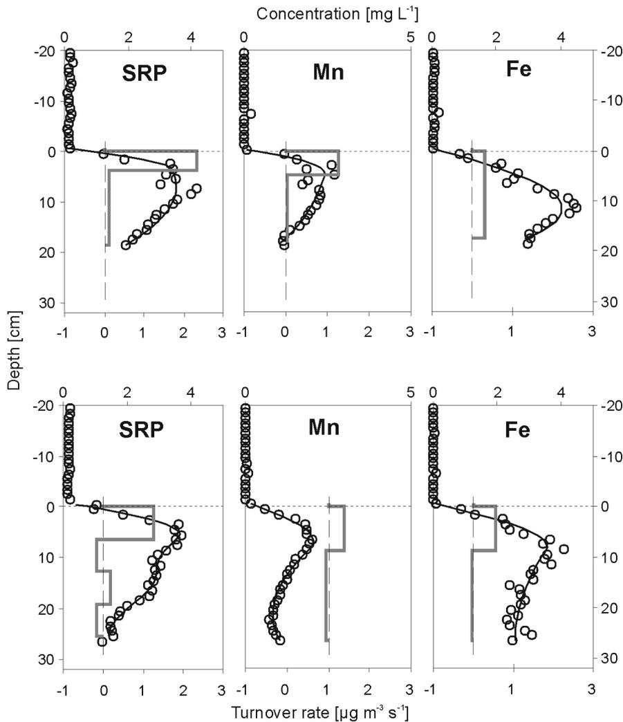
**Fig. 4.** Pore water concentration profiles of SRP, dissolved Fe, and dissolved Mn for two sampling locations (upper row: west located dialysis sampler, lower row: east located dialysis sampler) taken in June 2003. The mobilization rates, the fixation rates, the smoothed graphs and the coefficients of determination  $R^2$  were calculated with the program Profile V 1.0 (Berg *et al.* 1998).
