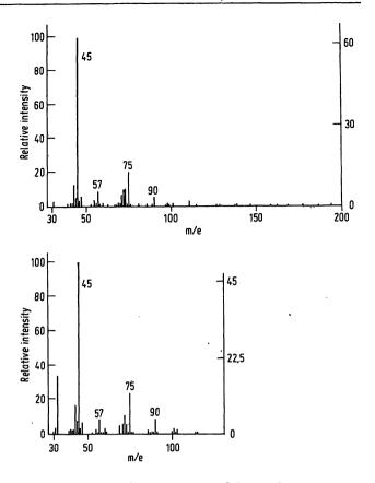
Fig. 2. Mass spectra of the compound of the gas chromatogram of figure 1 with relative retention time of 0.62 (top) and of authentic 2,3-dihydroxybutane (bottom). Cleavage of the  $C_2-C_3$  bond produces the base peak at m/e 45. Peaks > 60 are magnified 10 times.
