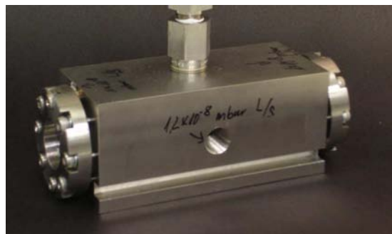
Figure 6.18.: Leek-tested gas-cell for measuring the interferometers nonlinearities.
