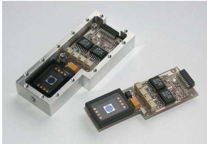
Figure B.4.: Photograph of the SMD quadrant photodiode electronics developed for the second experimental setup. The windows of the quadrant photodiodes were removed for the measurements.
