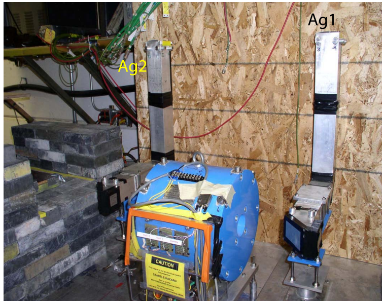
Figure 2.25: Picture of the gamma table showing the aero-gel counters (Ag1, Ag2) and the photon analyzing magnet
