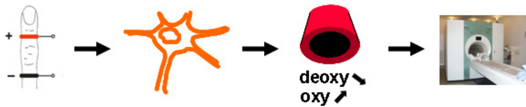
Figure 4: Signal cascade in functional magnetic resonance imaging (fMRI): An external stimulation leads to a neuronal activation in distinct brain areas which alters the metabolism, blood flow and blood volume in that area. These parameters affect the concentration of [deoxy-Hb] and [oxy-Hb] which determines the BOLD fMRI signal.
