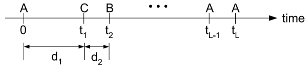
Figure 1: A non-equidistant time series with discrete symbols. The series consists of symbols A, B and C that occur at time 0, \dots, t_L . The delay between two successive symbols is denoted by d_k .
