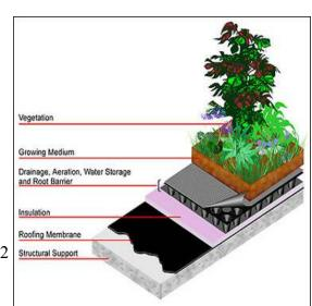
varies from system to system. As seen in the image to the right, typical greenroof gardens have the following layers: waterproofing or roofing membrane; drainage; growth medium; and vegetation. Flat roofs with a pitch less than five degrees often have an extra layer to drain excess water. Types of vegetation are dependent on the locality of the garden and the depth of the growing medium, or soil.
