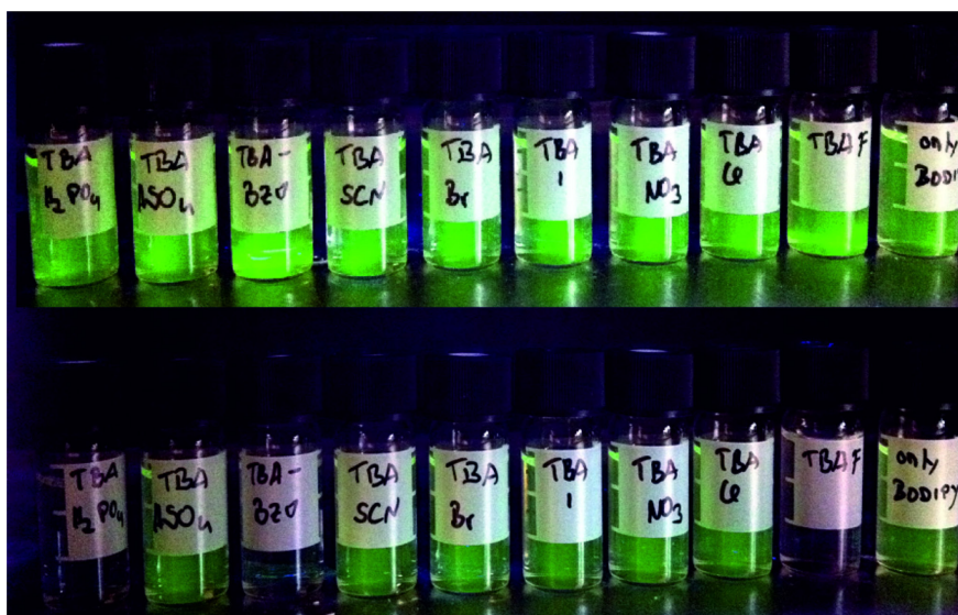
Figure 12 Visible response of 5 to various anions under UV-light a) in EtOH–H 2 O b) in MeCN.
