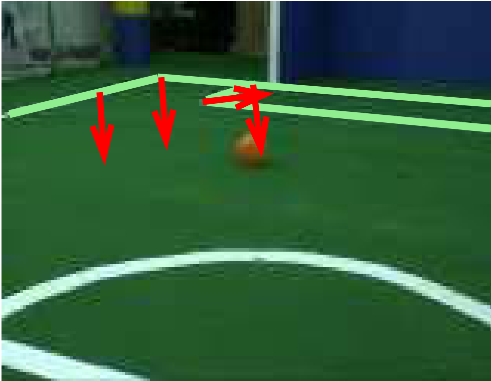
Figure 5.21: Field lines and corners. Green lines: detected field lines. Note that the center circle was successfully excluded. Red arrows: the starting points mark the corner locations. The heading marks the corners directions.
