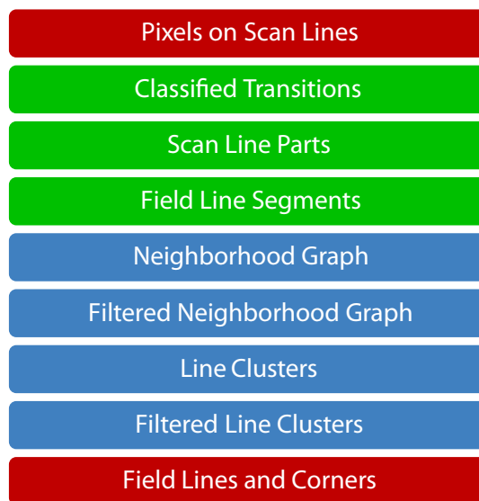
Figure 5.2: Sequence of representations . All representations used while detecting field lines. The source representation is pixels on scan lines. The target representation is field lines and corners, relative to the robot. The first three representations (green background) are scan-line based. This means only vertical relations of pixels and detected objects are used. Starting from the fourth representation (blue background) horizontal relations are also taken into account. This distinction is important when the complexity of the system is analyzed. The subsections in this section describe how the representations shown are calculated in this sequence.
