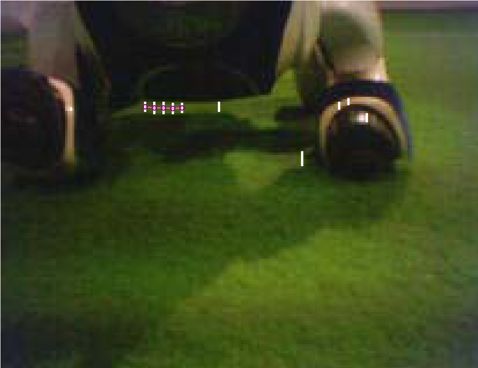
Figure 5.15: Filtered neighborhood graph containing edges that cover parts of an image without a field line. This is a very rare case. However, it does not cause the creation of a false field line percept, as no line cluster is created (cf. section 5.1.8).
