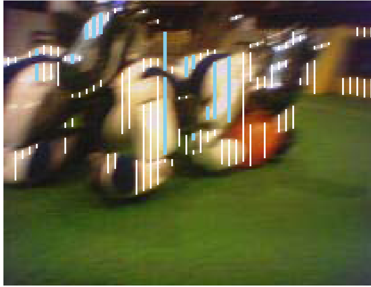
Figure 5.8: Conditions to remove false positives. Condition 1: The line segment width decreases towards the horizon. The sky-blue segments are longer than another segment below on the same scan line. This is why they are removed by C_1 .
