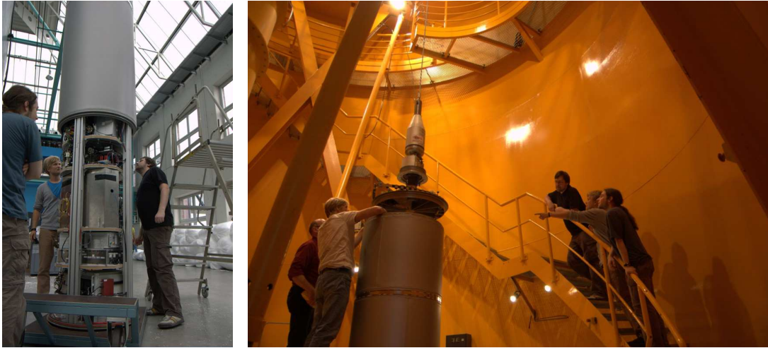
Figure 5.1: Final check of the QUANTUS-I payload by the science team 2 , which is usually done in the integration hall before hand-over to the drop tower operators (left). Closing of the capsule with an upper shell and preparation for lift-up with a winding mechanism is done by the operators (right).
