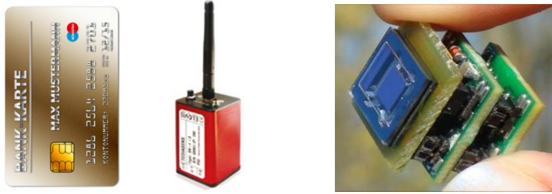
Fig. 15: A commercial wireless sensor node with a 3D acceleration sensor, 802.11g radio, 138 meters communication range, size 40x40x82 mm 3 , weight 220 grams with accumulator and antenna 36 ( left ). A custom wireless sensor node with a temperature sensor, powered by a piezoelectric vibrational energy harvester and built from of-the-shelf components. The system is fully autonomous and generates sufficient power to measure and transmit the environmental temperature with an interval of fifteen seconds ( right ) [Loc13].
