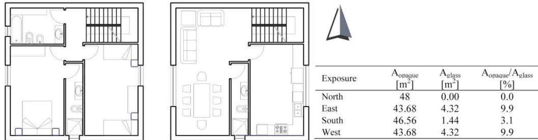
Fig. 3. Geometric characteristics and planimetries assumed for the house examined on 2 communicating levels through an interior staircase.
