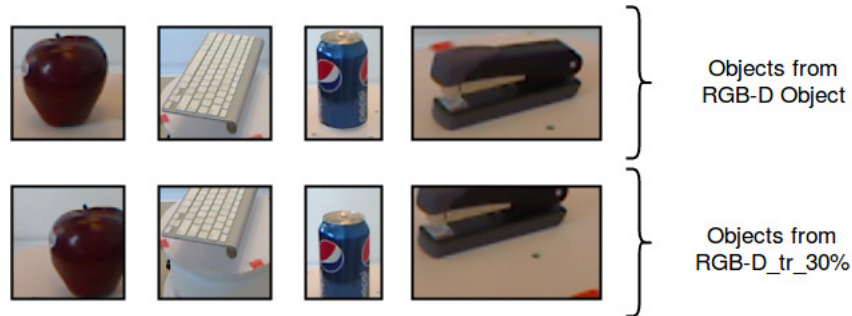
Fig. 3: Original crops from the RGB-D Object dataset (top) and the same crops after random translations (bottom)
