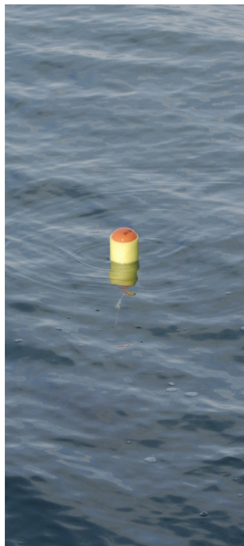
Figure 2: Drifter MD03i with only approximately 0.08 m above the water surface.
