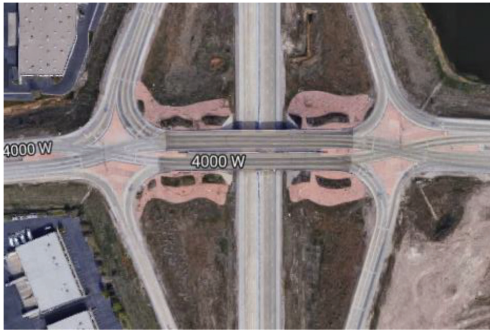
Figure 2.2 Diverging diamond interchange.
