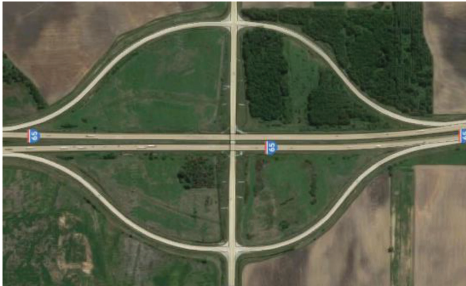
Figure 2.1 Conventional diamond interchange.
