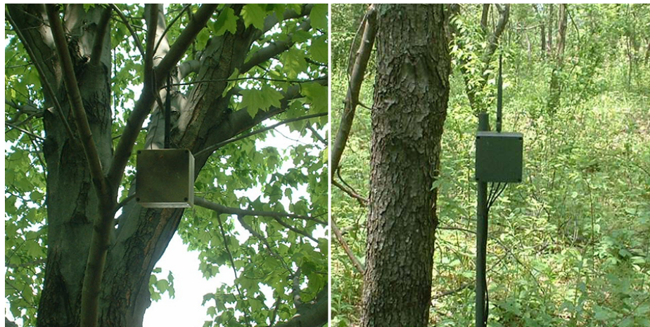
Figure 3.2. Examples of node configurations in the ASWP testbed. A node hanging from a tree without external sensors (left) and a node mounted onto a PVC pipe with external sensors attached (right).
