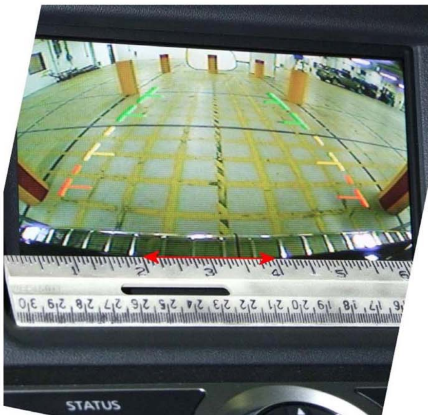
Figure 14. Field of View and Image Quality Assessment Photo for the 2010 Nissan Murano
