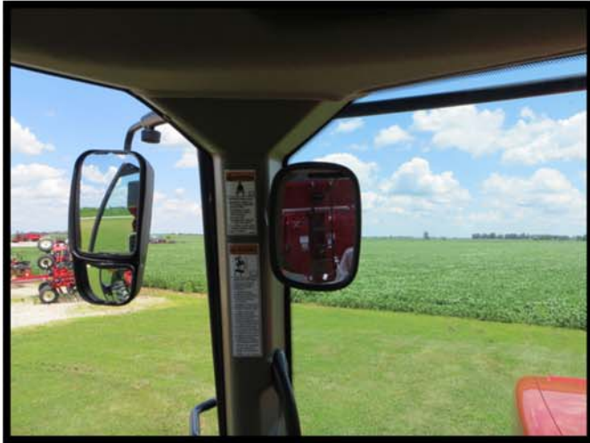
Figure 5.37. Case IH Magnum 310 dual stacked extended-arm mirror view of rearward visibility test grid.
