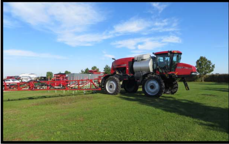
Figure 5.60. Case Patriot 4430 Self-Propelled Sprayer with 36.6 m (120 ft.) booms adjacent to rearward visibility test grid.
