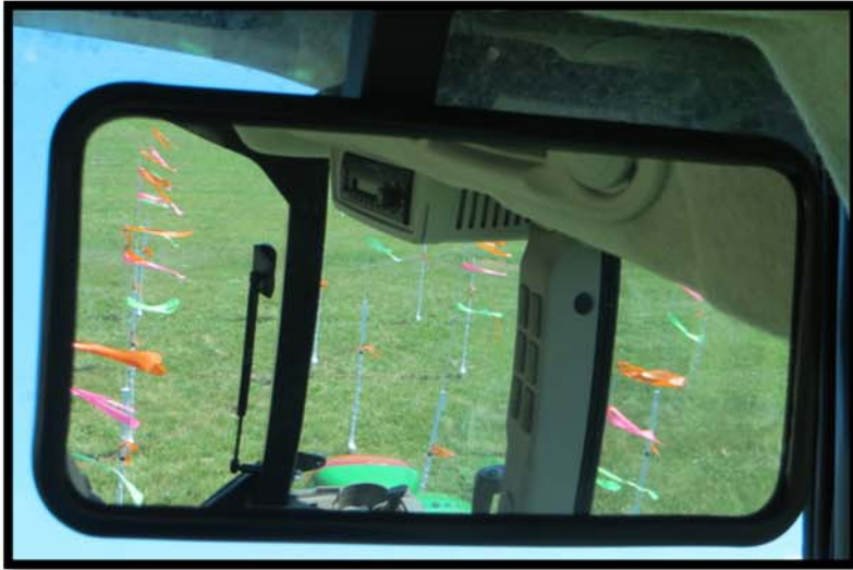
Figure 1.6. Interior tractor mirror with cab component obstructions.
