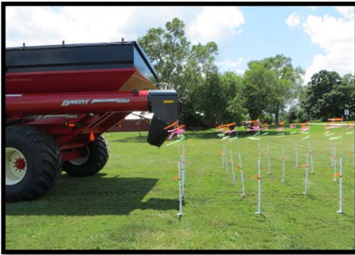
Figure 5.29. Case IH Magnum 310 with Brent 1082 grain cart in tow positioned adjacent to rearward visibility test grid.
