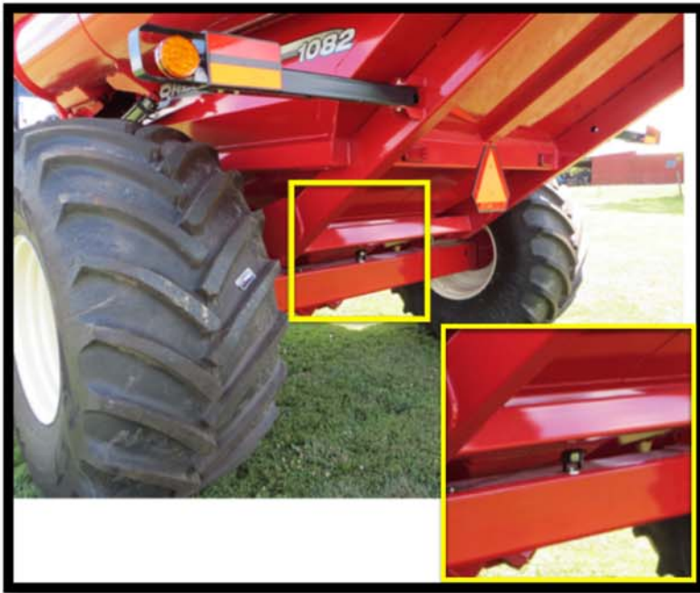
Figure 5.34. Case IH Magnum 310 with Brent 1082 grain cart, central frame cross member camera mount location.
