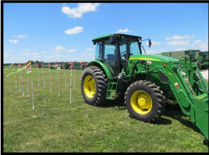
Figure 5.38. John Deere 6140D MFWD mid-sized tractor positioned adjacent to rearward visibility test grid.
