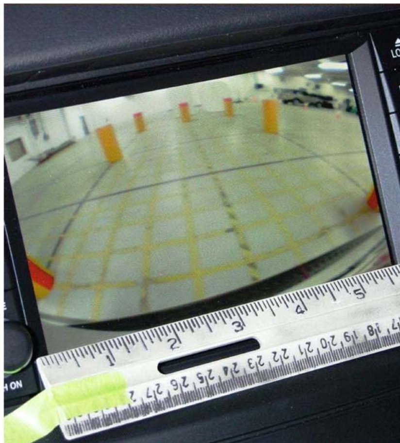
Figure 11. Field of View and Image Quality Assessment Photo for the 2010 Dodge Grand Caravan
