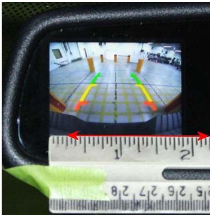
Figure 12. Field of View and Image Quality Assessment Photo for the 2010 Ford F150
