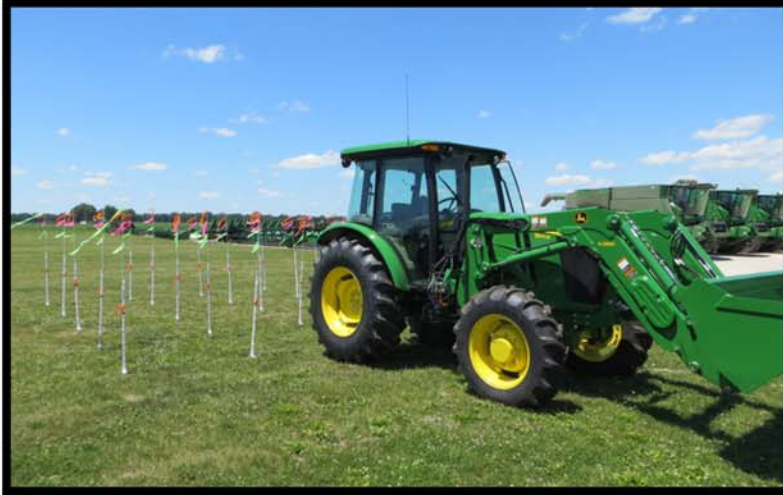
Figure 5.46. John Deere 5100E utility sized tractor positioned adjacent to rear visibility test grid.
