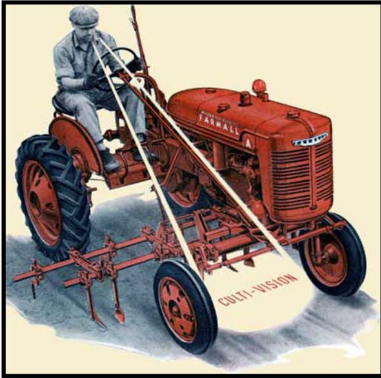
Figure 4.1. Farmall A featuring Culti-Vision; Offset frame design allowed for increased operator view of the specific task (Antique Farming, 2016).
