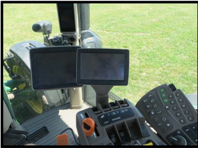
Figure 5.28. John Deere 8360R—OEM monitors mounted to control arm and front cab pillar.
