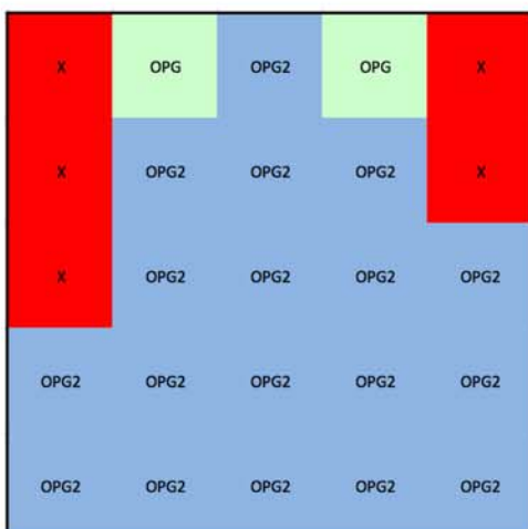
Figure 5.44. John Deere 6140D—Best union of all viewing mediums rearward visibility test grid results.
