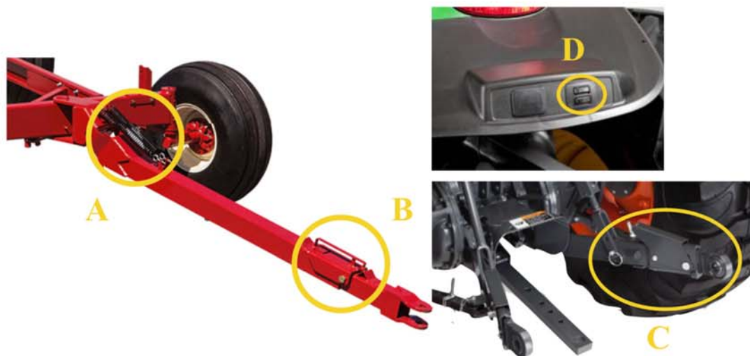
Figure 6.8. Hitching assistive devices—A. spring assisted tongue, B. telescoping tongue, C. telescoping tractor lift arms, D. fender mounted lift arm controller.
