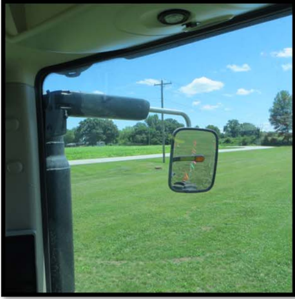
Figure 4.5. Right extended-arm mirror view of assessment grid from operators' forward facing position.
