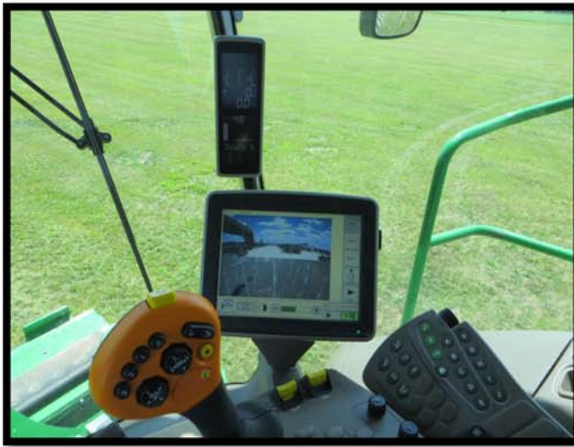
Figure 5.59. Factory monitor utilized for camera display.
