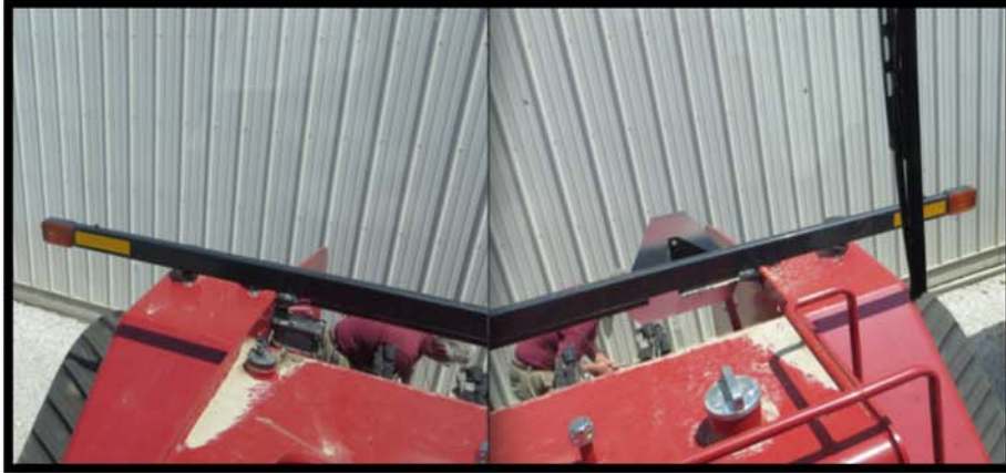
Figure 1.2. Driver's view of assistant at hitching point with full seat rotation in both directions.
