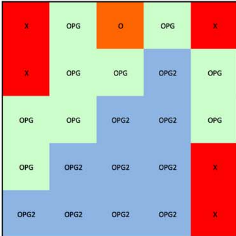
Figure 5.10. Case IH Quadtrac 420—Union of all equipped mirrors rearward visibility test grid results.
