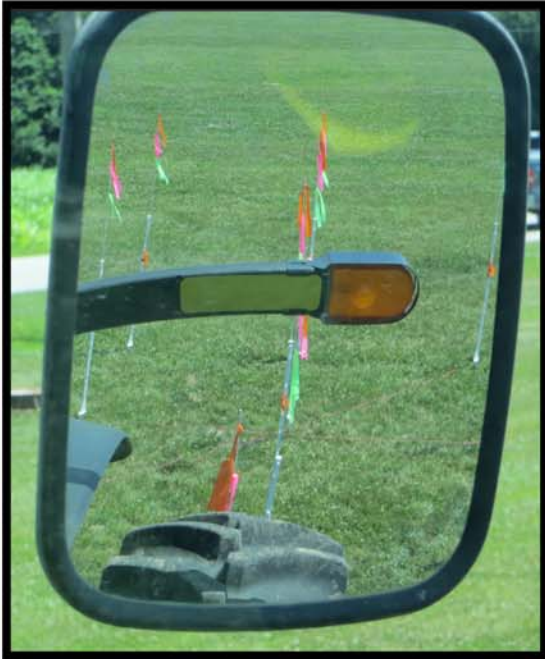
Figure 4.6. Full view optical zoom of right extended-arm mirror from operators' forward facing position.
