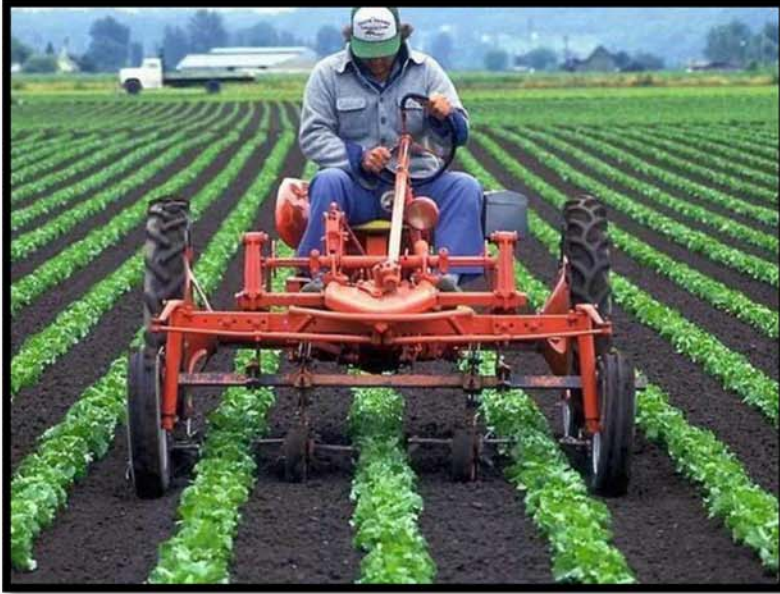
Figure 1.1. The open-frame design of the Allis Chalmers model G allows a nearly unobstructed view of the specific task (source: Delaware, 2010).
