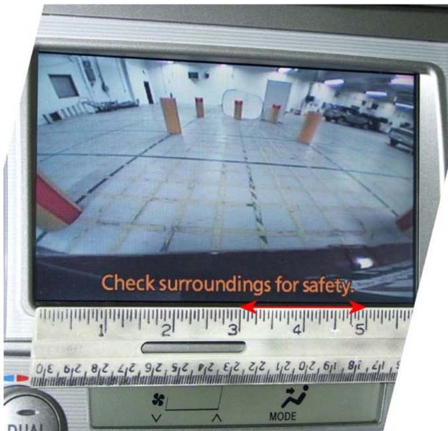
Figure 15. Field of View and Image Quality Assessment Photo for the 2011 Toyota Camry
