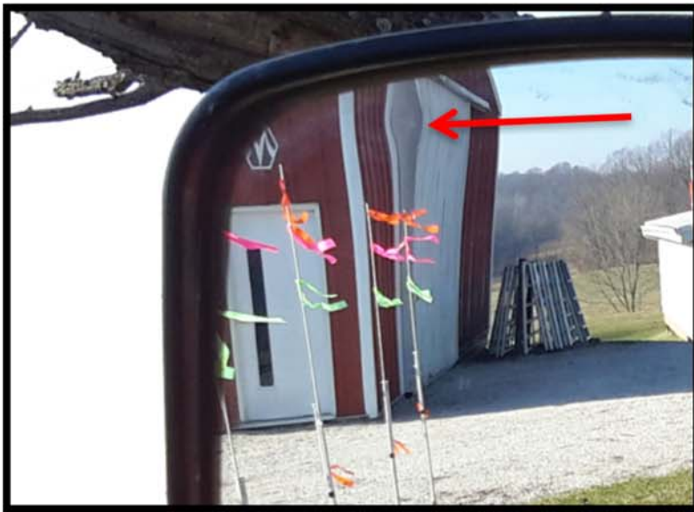
Figure 1.5. Distortion caused by convexity of the mirror surface.
