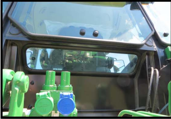
Figure 5.45. John Deere 6140D—Low rear cab window for improved direct viewing of hitch area.
