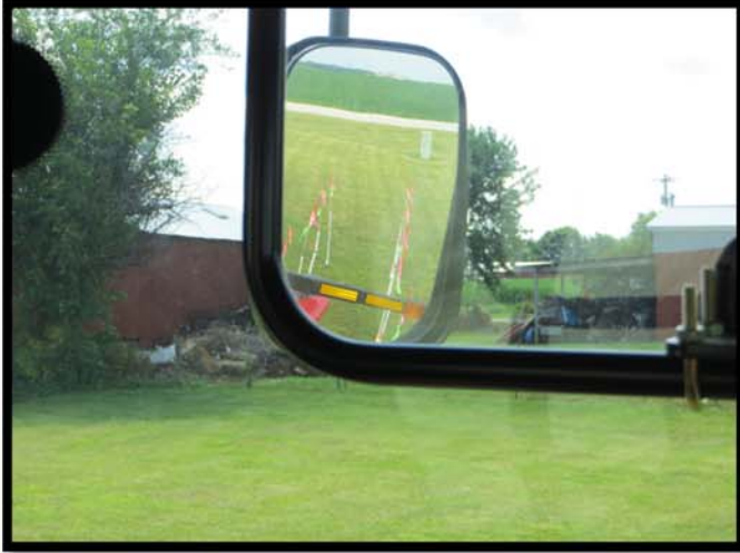
Figure 5.4. Case IH Quadtrac 420—Right extended-arm mirror view of rearward visibility test grid.
