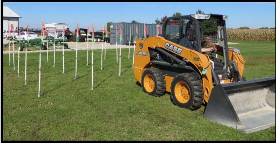
Figure 5.69. Case SV185 skid-steer, mid-sized 840 kg (1,850 lb.) operating load positioned adjacent to rearward visibility test grid.
