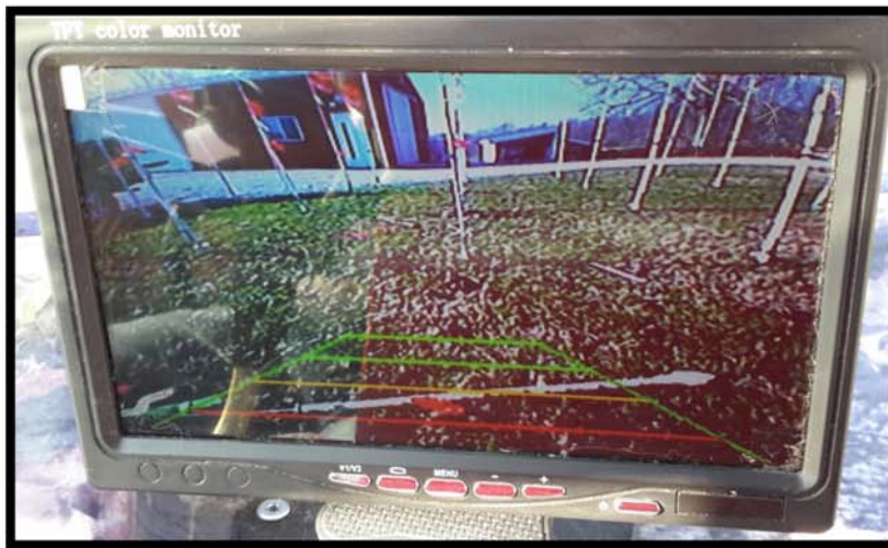
Figure 5.78. TFT dual input, 17.8 cm (7 in) color monitor paired with 170° waterproof camera with overlaid distance estimating grid.
