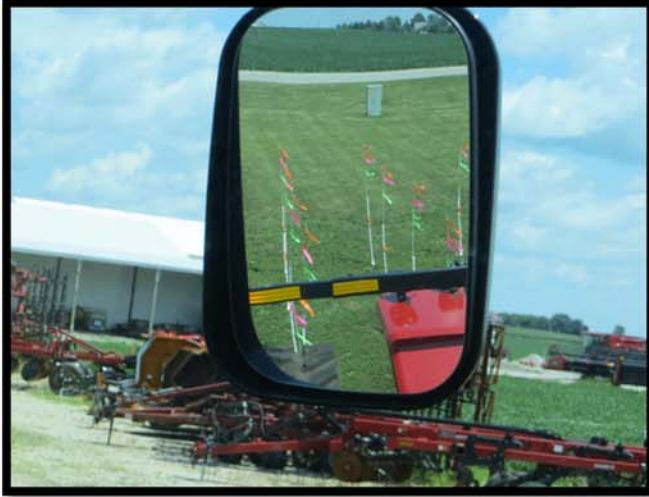
Figure 5.6. Case IH Quadtrac 420—Left extended-arm mirror view of rearward visibility test grid.
