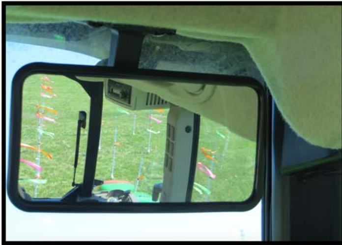
Figure 5.47. John Deere 5100E—Interior mirror with impeding cab components view of rearward visibility test grid.
