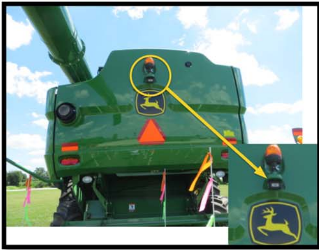
Figure 5.55. John Deere S660 combine—Optional camera location.
