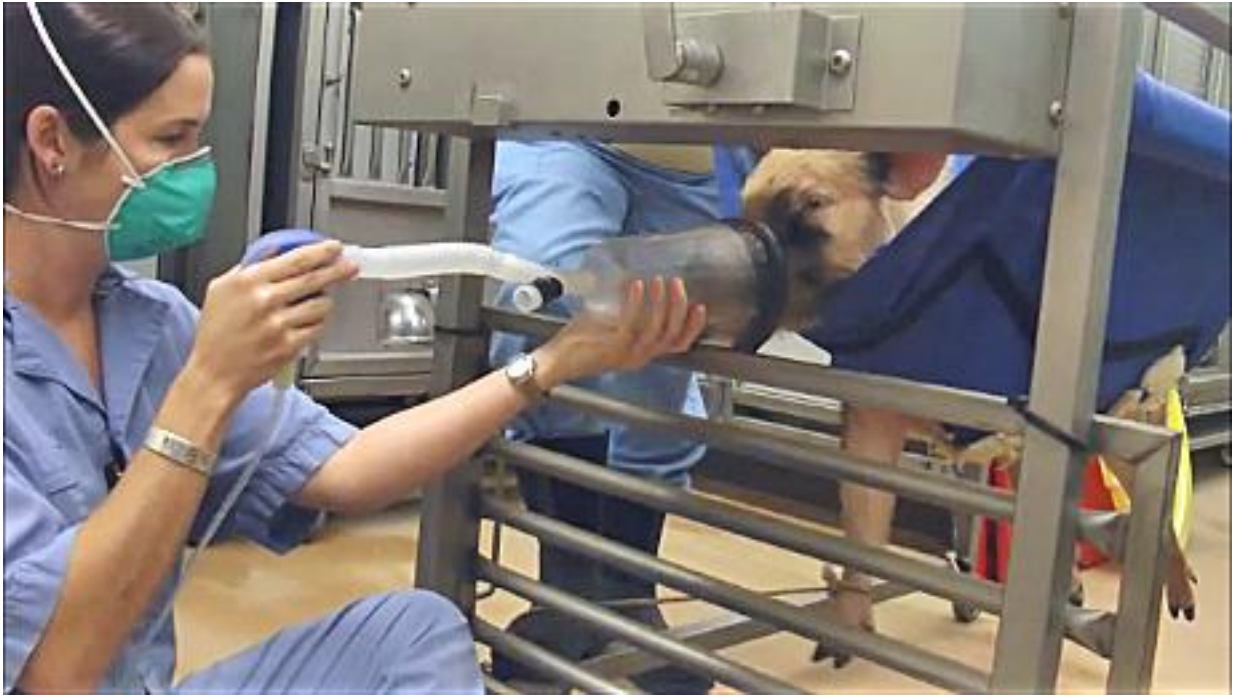
Figure 4.1: Photo depicts the sling-restraint apparatus. Each pig is acclimated to the sling and trained to breathe normally through a standard nose cone.
