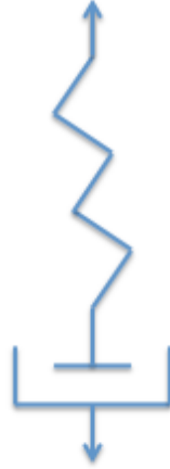
Figure 1. Maxwell Model for creep.
