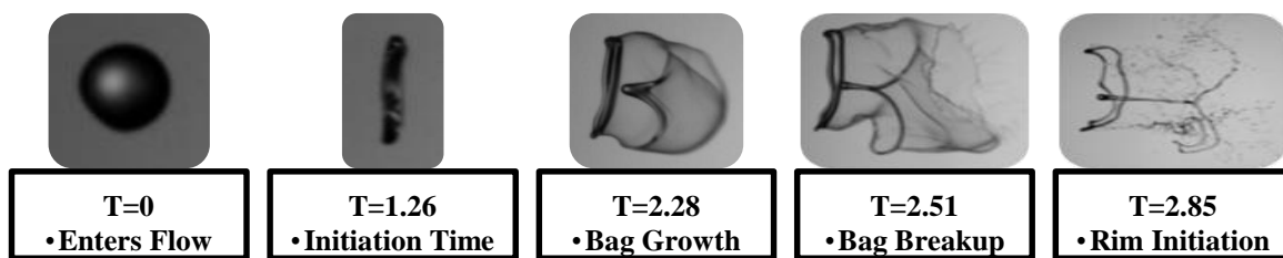
Figure 4.9. 0.8% CMC-7MF ( n=0.93 , K=0.046 ) in the Bag and Stamen Breakup Regime, We=21 . d_0 = 2.75mm ; L_{Bag} = 13.3mm
