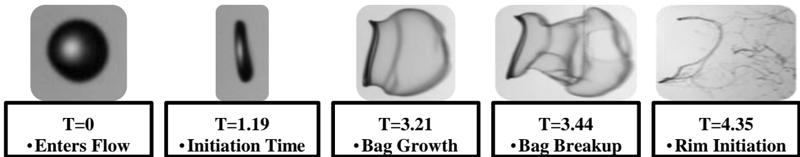
Figure 4.7. 84.96% Gly/0.05% CMC-7MF ( n=0.88 , K=0.30 ) in the Bag Breakup Regime, We=27 . d_0 = 2.53\text{mm} ; L_{Bag} = 13.6\text{mm}
