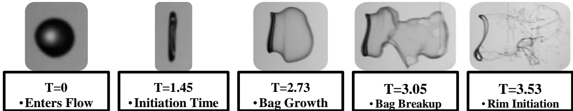
Figure 4.5. 74.96% Gly/0.06% CMC-7MF ( n=0.90 , K=0.13 ) in the Bag Breakup Regime, We=21 . d_0 = 2.54\text{mm} ; L_{Bag} = 18.8\text{mm}
