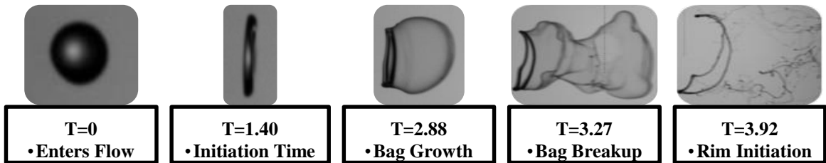
Figure 4.6. 79.95% Gly/0.06% CMC-7MF ( n=0.89 , K=0.20 ) in the Bag Breakup Regime, We=24 . d_0 = 2.51\text{mm} ; L_{Bag} = 17.9\text{mm}
