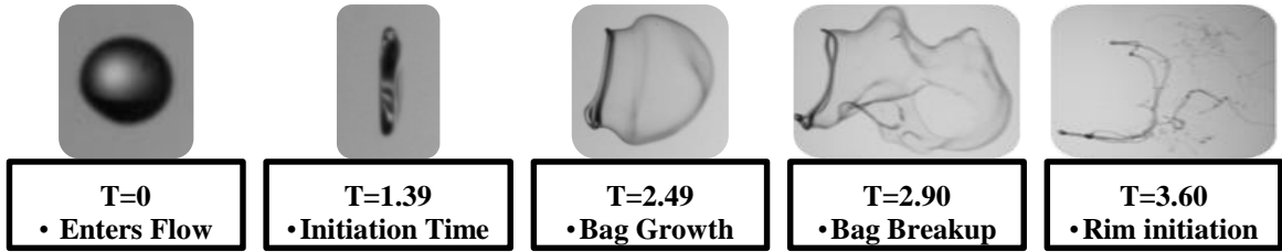
Figure 4.4. 0.5% CMC-7HF ( n=0.71 , K=0.37 ) in the Bag Breakup Regime, We=20 . d_0 = 2.72\text{mm} ; L_{Bag} = 20.2\text{mm}
