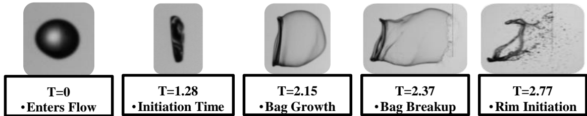
Figure 4.1. DI-Water ( n=1.00 , K=0.00094 ) in the Bag Breakup Regime, We=15 . d_0 = 2.64mm ; L_{Bag} = 12.78mm
