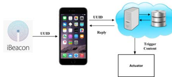
Figure 2.3. Working principal of the beacon
