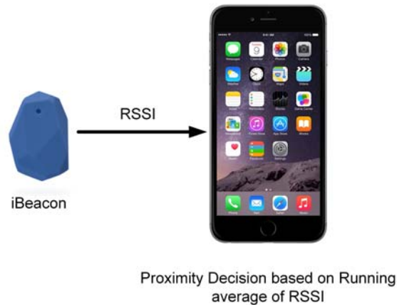
Figure 4.1. Current approach used by Apple's CoreLocation Framework.
