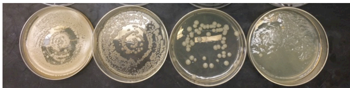
Figure 4.4. V. harveyi after exposure to UV radiation at 289 nm at the same dilution with increasing dose from left to right (0 mJ/cm 2 , 13 mJ/cm 2 , 26 mJ/cm 2 , 33 mJ/cm 2 ).
