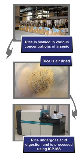
Rice was soaked in water containing arsenic, air dried, and then prepared and analyzed for changes in arsenic concentration using ICP-MS.
