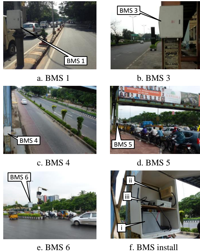
Fig 2 Bluetooth Monitoring Stations ((a) – (e) shows the BMS at different locations. (f) shows a typical BMS with (i) battery to supply power, (ii)13dbi antenna and (iii) host machine)
