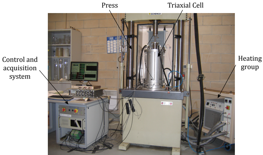
Figure 4.2: Triaxial test set-up.
