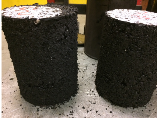
Figure 3.4: Overcompaction problem in the gyratory compactor.
