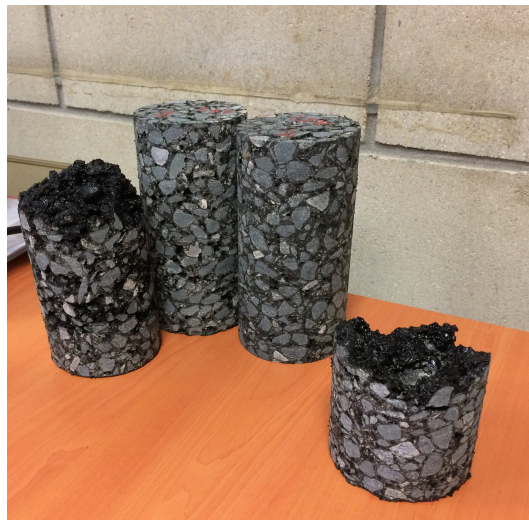
Figure 3.3: Samples with different bitumen content.
