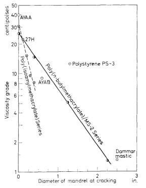
Figure 1. Brittleness of films at  $70^{\circ}$ F and 50 per cent relative humidity as a function of their viscosity grade (1.5-mil thick films on 1-mil aluminium foil).
