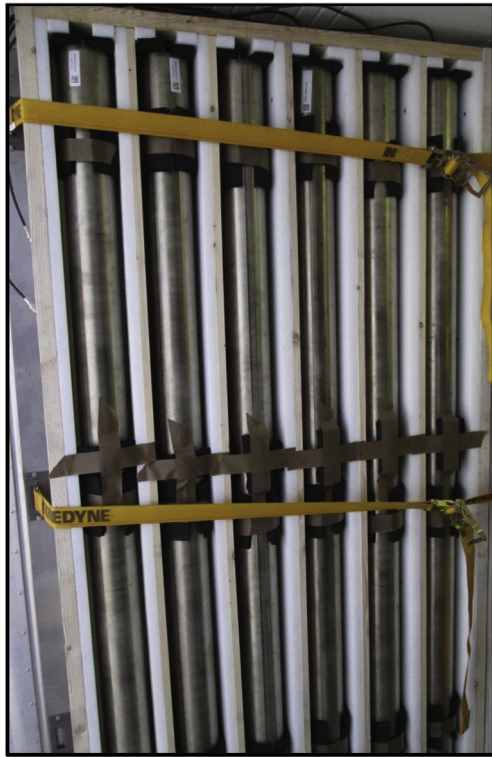
Fig. 3. Interior view of one of the \text{BF}_3 modules with the inward-facing moderation removed.
