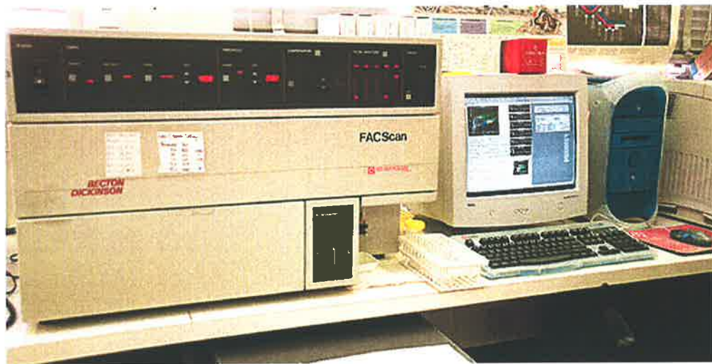
Photograph 2-5: Becton Dickinson's FACScan. The channel frequencies were: FL1 - Excitation: 495nm; Emission: 510nm. (FITC) FL2 - Excitation: 565nm; Emission: 575nm. (PE) FL3 - Excitation: 470nm; Emission: 677nm. (7-AAD)
