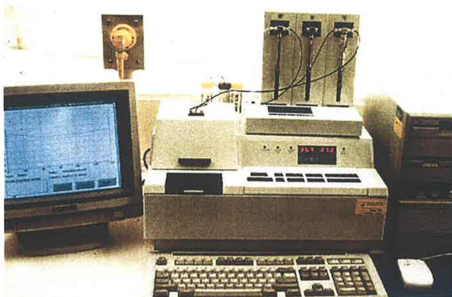
Photograph 2-4: Luminometer Model 1251 from Biorbit Oy, Turku, Finland. The sample tubes were inserted in a carousel, and the luminometer pump automatically injected 0.5ml of lucigenin per tube. Chemiluminescence (in mV) was continuously recorded.
