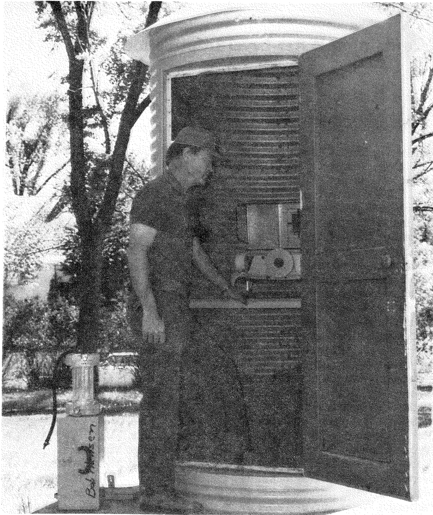
Bob Hansen, basic-data supervisor with the Conservation and Survey Division, gets ready to make a water-level measurement.
