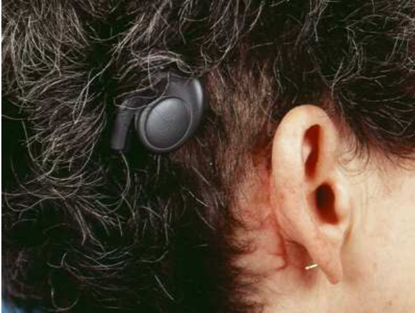
Figure 3: Externally worn DACS audio processor attached to the percutaneous plug. Sounds are received by the microphone signal processed and transmitted to the implanted DACS transducer via the percutaneous plug.
