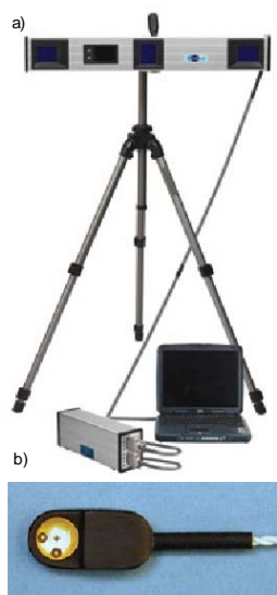
Figure 2.1 : Codamotion system a) sensors unit; b) small infrared light emitting diodes markers.
