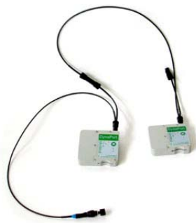
Figure 2.24: MiniMod system (DynaPort) with two inertial modules.
