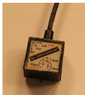
Figure 2.18: Tri-axial accelerometer and tri-axial gyroscope including conditioning module.
