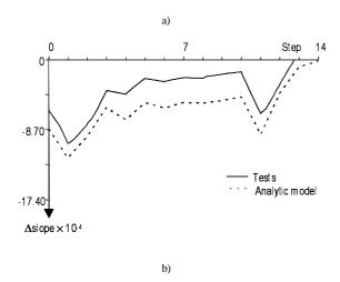
Figure 17: Prediction and measurement: of  $\Delta$ slope (Eq. 1) with iteration step : (a) single point load, Load case 15 and, (b) double point load, Load case 23
