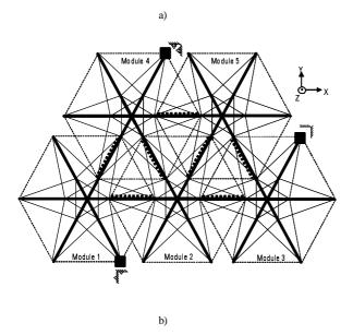
Figure 2: Plan view: (a) three module structure— symmetric configuration (Fest et al. 2003), (b) five module structure— asymmetric configuration, note that Module 2 and Module 5 are not supported.
