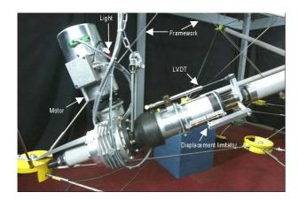
Figure 10: Elevation view of an actuator set in a strut. Note the LVDT and the displacement limitator
