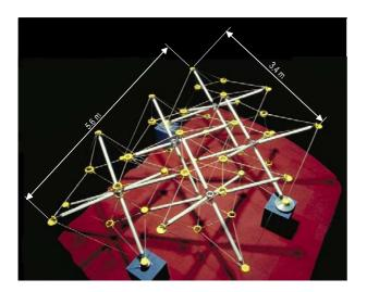
Figure 1: Picture of the five modules without actuators showing the three supports. Note that between modules, compression elements do not touch, that two modules are not supported and that the configuration is asymmetric.
