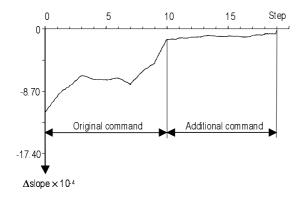
Figure 19: Iterative slope compensation, load case 8
