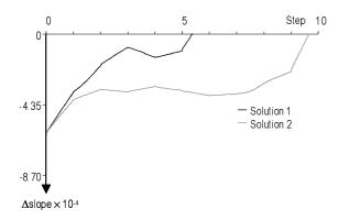
$Figure \ 18: \hspace{1.5cm} Slope \ compensation \ evolution \ comparison \ between \ two \ equivalent \ quality \ solutions, \ load \ case \ n^\circ 14$
