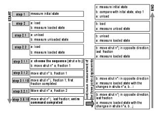
Figure 12: Testing procedure
