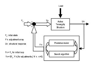
Figure 5: Shape control loop (Fest et al. 2003)
