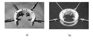
Figure 4: Two stages of the connection module joint: (a) three module structure open ring (Fest et al. 2003) and (b) five module structure closed ring
