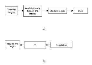
Figure 6: Relations between the length of the telescopic members and the structure shape: (a) transformation from given structural geometry to slope (b) transformation from target slope to required structural geometry.
