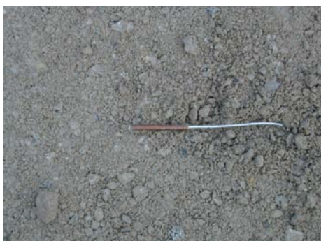
Temperature probes PT100 at -26cm. Left: detail of the probe. Right: HMF laying. Probes were protected with a fine bituminous layer.
