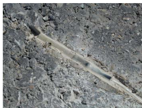
Temperature probes located at the HMF – HMT interface (-12cm). Probes were fitted with silicon.
