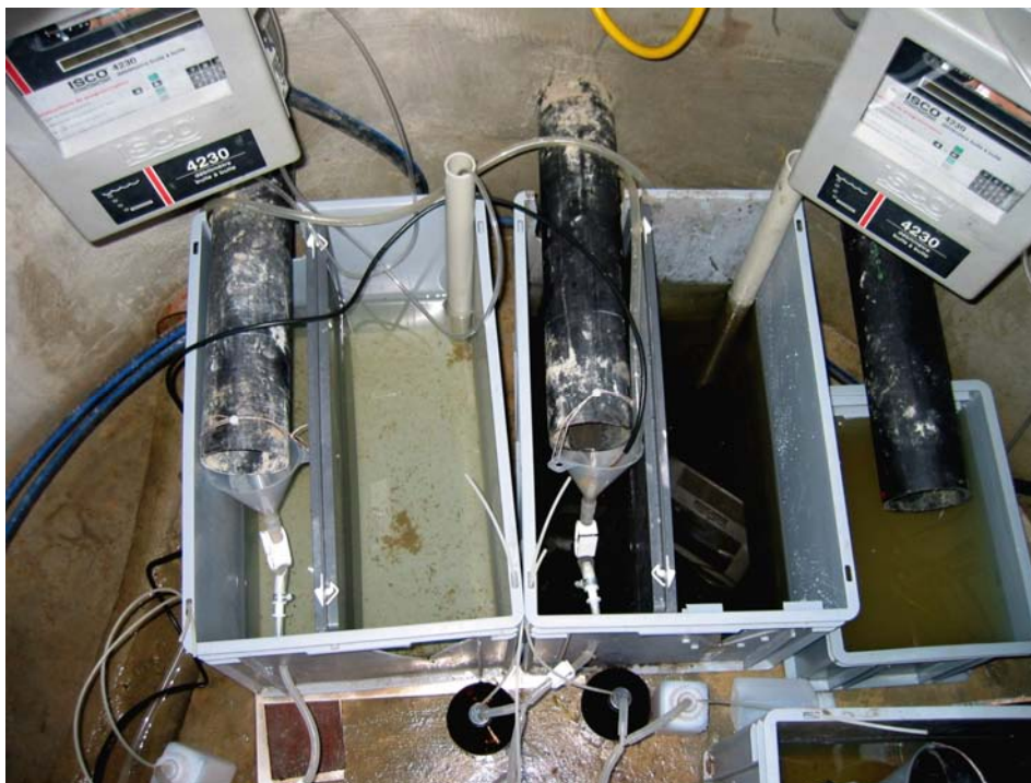
Figure V.3: illustration of the collecting pipes and weirs. From left to right are visible the LW, road runoff (note the water colour!) and SH pipes and weirs. Far bottom right is discernable the LH collecting pipe. Grey boxes are the flowmeters. Note that the air pipes are placed in tubes to avoid the effect of waves forming at the surface of the weirs. Are also visible the funnels and bottles collecting the first-flush. At last, in the runoff funnel is placed the EC probe (black cable).
