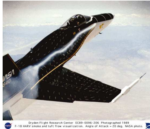
Fig. 7.3: A NASA F-18 at 20 degrees angle of attack. The strake vortex has been made visible with smoke showing the vortex breakdown which occurs toward the trailing edge of the wing. Courtesy of NASA: http://www.dfrc.nasa.gov/gallery/photo/ .
