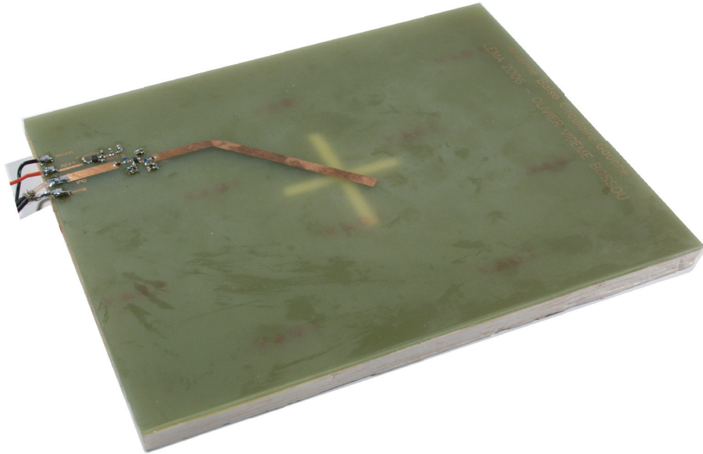
FIGURE 4.17: The LNA printed with the feed line
