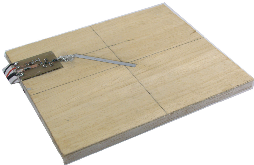
FIGURE 4.18: The LNA glue on the ground plane
