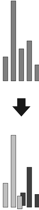
Fig. 1. Example of “cut” of a bunch originated by two temporally close traces. A 5-sample bunch is cut into two 3-sample ones.
