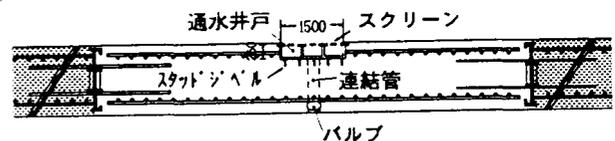
Fig.8 Well structure installed RC diaphragm wall
