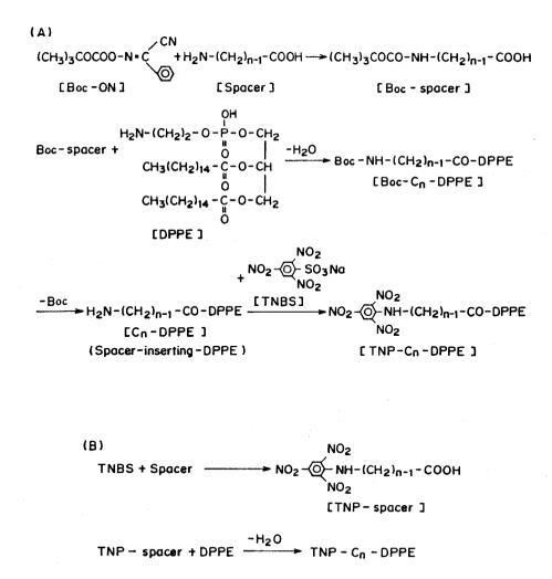
Fig. 1. Schematic diagram of reaction principle. (A) is our method and (B) is conventional one.
